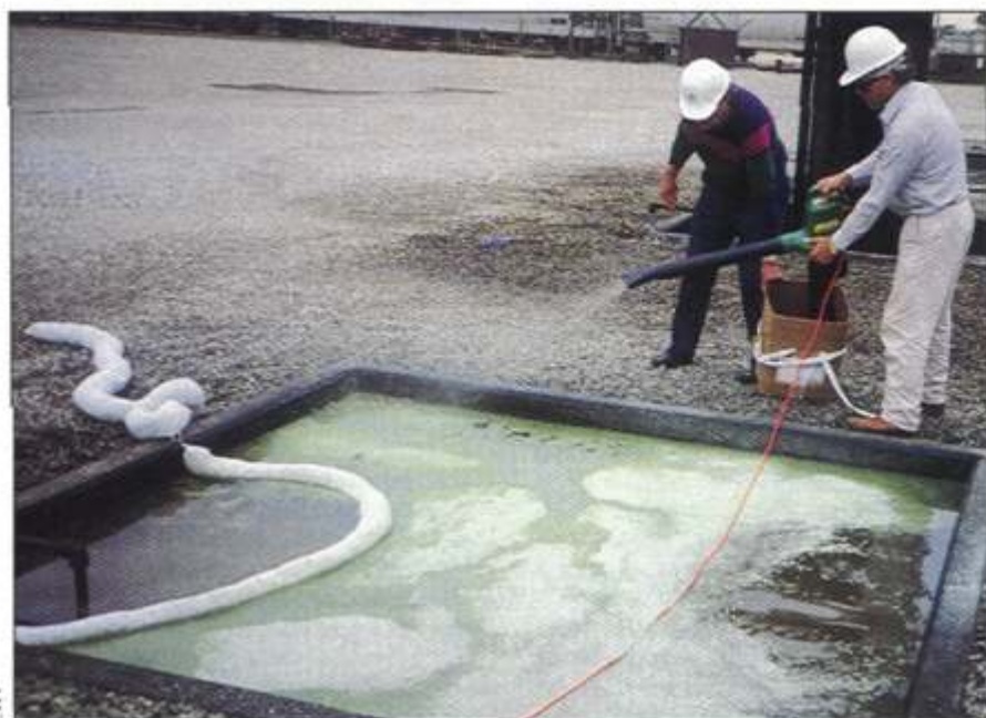
LWT Executive Vice President Bill Gannon, right, sprays particulate Solidifier™ on oil-contaminated water at a recent demonstration.
