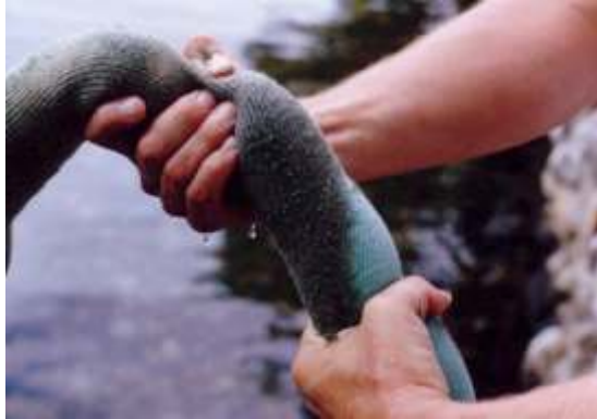
SPI Oil-Bond™ Boom after being absorbed and solidified with Diesel Fuel.
