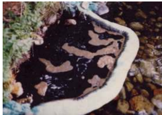
The SPI Oil-Bond™ Boom is wicking in the oil, while containing the oil spill from spreading
