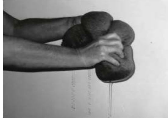
Typical oil only sorbent boom fully saturated with Diesel Fuel, squeezed lightly.
